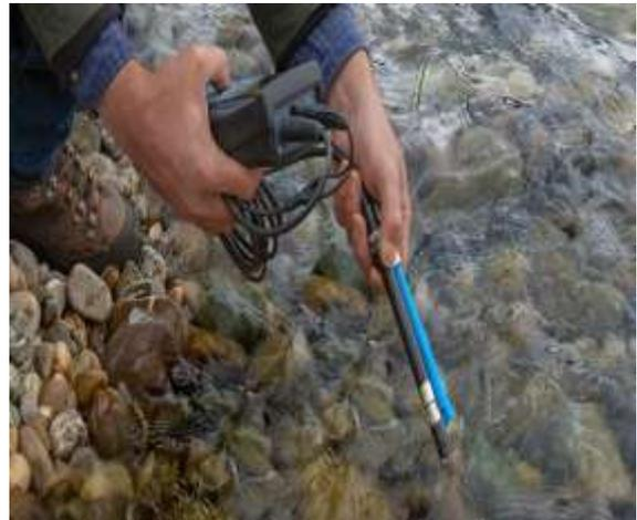
Figure 3. Portable Portal Transmitter to determine the electrical conductivity of water
